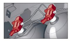
► Each gas tank is equipped with its individual cylinder valve and manual stopcock.
